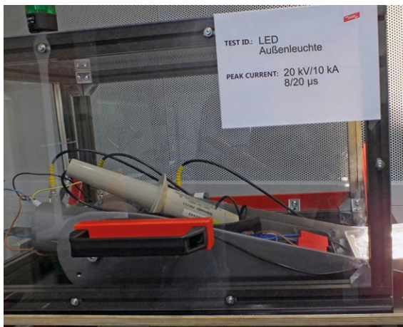
Figure 7 Test setup for a complete LED street lighting system in the laboratory
